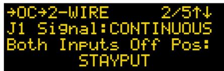
As of firmware version 3.8.1 this screen allows for different types of control signals to be applied to the J1 port. That is set with the second line of this screen. The options for the J1 Signal type are:
